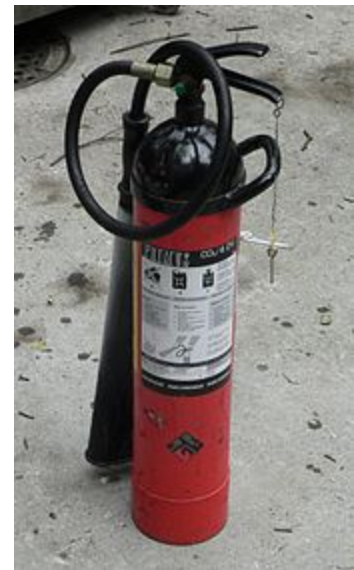
A carbon dioxide fire extinguisher rated for flammable liquids and gasses
